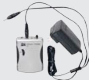
Amigo T5 comes with a wall charger that can charge 2 units simultaneously.
